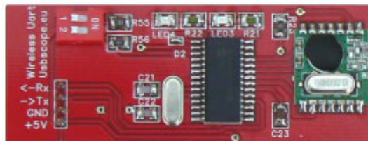
Figure 3, Wireless UART with PIC/AVR interface
